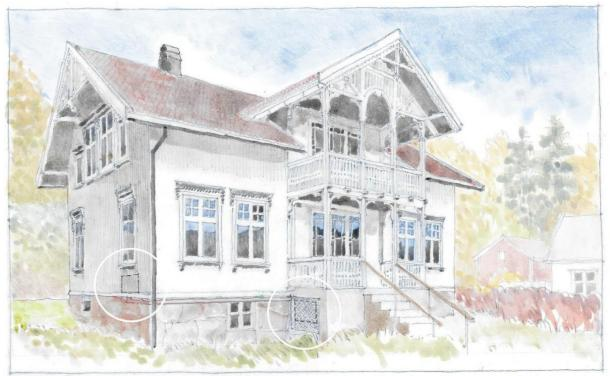
The third solution is to lay the ducting under the drip board along the facade and around the corner. On the short side of the house, there is a floor-mounted indoor unit that means one avoids having to lay the ducting all the way up the facade. Photo: Romfarer Arkitekter AS/Stein Høglund
